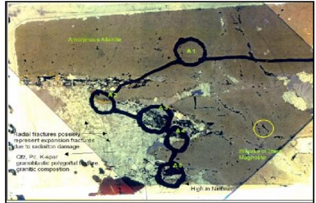
Fig. 5 Photomicrograph of polished thin section of allanite scale width 2.5cm, Circles, A<sub>1</sub>-A<sub>5</sub> Minerals probed
