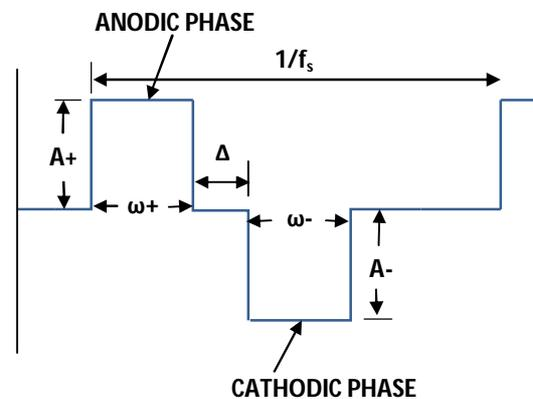
Fig.2 The biphasic stimulation current waveform
