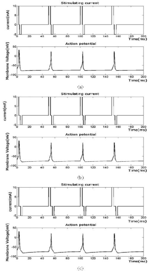
**Fig.6** Biphasic stimulating current and the action potential evoked by varying the IPG (a)  $\Delta = 1\text{ms}$  (b)  $\Delta = 2\text{ms}$  (c)  $\Delta = 3\text{ms}$ .
