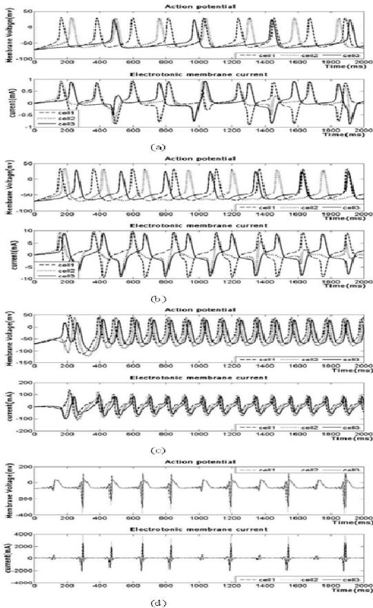
**Fig.5** Action potentials of three cell compartments and the electrotonic current flowing through their cell membranes for the given values of stimulating current  $I_{stim} = [6 \ 4 \ 2]$  and different values of gap conductances with  $G_1 = G_2$ . (a)  $G_1, G_2 = 0.01$ , (b)  $G_1, G_2 = 0.1$ , (c)  $G_1, G_2 = 1$ , (d)  $G_1, G_2 = 10$ .
