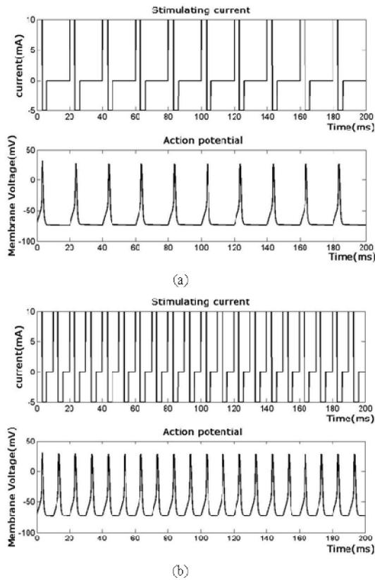
**Fig.9** Biphasic stimulating current and the action potential developed by increasing stimulating frequency.
