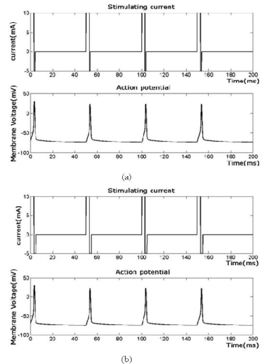
**Fig.7** Biphasic stimulating current and the action potential produced with non-uniform pulse duration.
