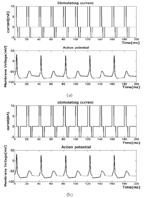
**Fig.10** Biphasic stimulating current and the action potential initiated by increasing stimulating amplitude and IPG for 50Hz frequency pulse.
