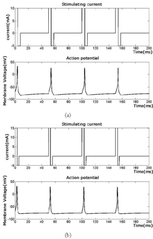
**Fig.8** Biphasic stimulating current and the action potential originated by increasing the pulse duration, cathodic pulse amplitude respectively.
