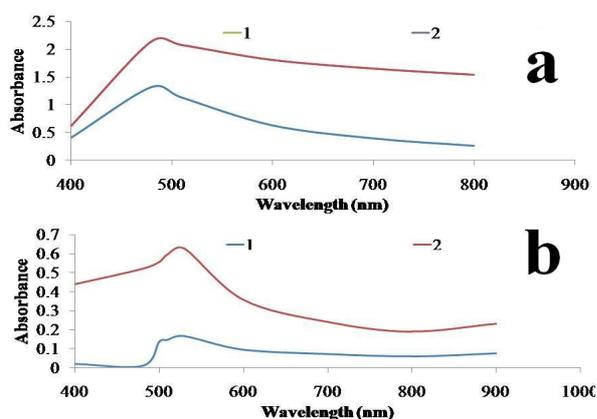
**Fig. 1** UV-Visible spectra of silver (a) and gold (b) nanoparticles synthesized by using the *F. oxysporum* f.sp. pisi.
