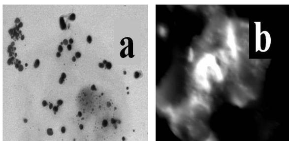
Fig. 2 (a) TEM and (b) SEM images of gold nanoparticles synthesized by using the *F. oxysporum* f.sp. *pisi*.
