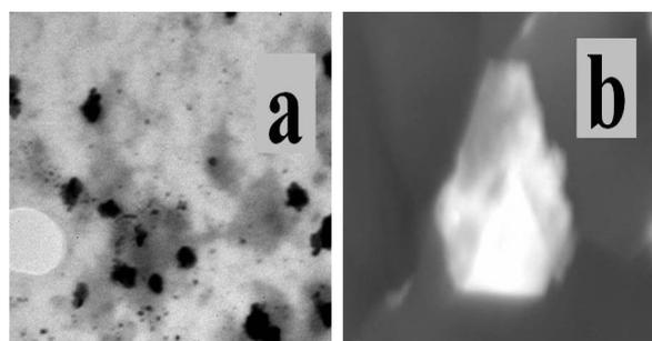
Fig. 3(a) TEM and (b) SEM images of silver nanoparticles synthesized by using the *F.oxysporum*f.sp.*pisi*
