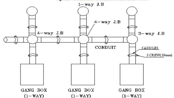
**Figure 3:** Layout diagram for circuit1
