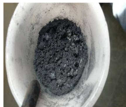
Figure 2a Spongy structure of expanded graphite after heat treatment
