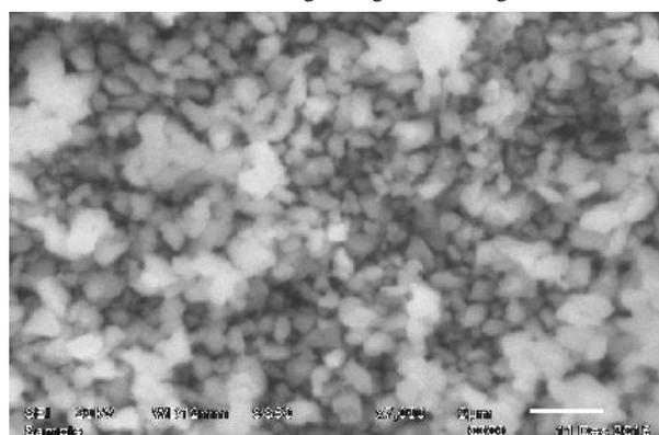
Fig. 3 SEM image of BiVO<sub>4</sub> Photocatalyst.
