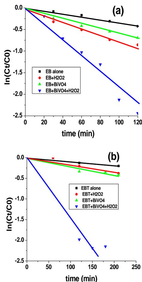
Fig. 7 Plot of lnCt/C<sub>0</sub> vs time for photodegradation study of (a) EB and (b) EBT
