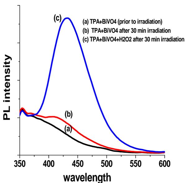
Fig.6 Photoluminescence spectra of TPA solution containing BiVO<sub>4</sub> in presence and in absence of H<sub>2</sub>O<sub>2</sub> before and after irradiation for 30 min.
