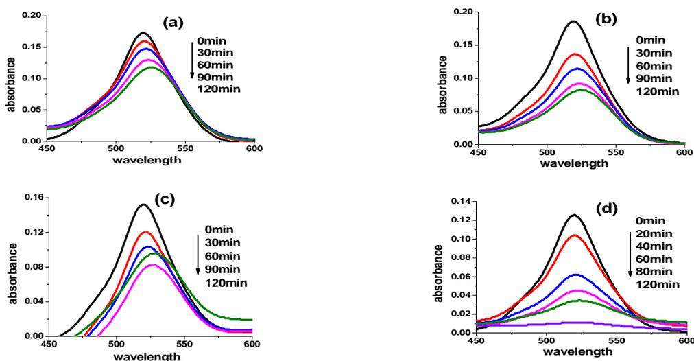
Fig.4 U.V-visible spectra of (a) EB aqueous solution, (b) EB+H<sub>2</sub>O<sub>2</sub>, (c) EB+BiVO<sub>4</sub> and (d) EB+H<sub>2</sub>O<sub>2</sub>+BiVO<sub>4</sub> as a function of irradiation time (EB-10ppm, BiVO<sub>4</sub>-100mg, H<sub>2</sub>O<sub>2</sub>-10μm)
