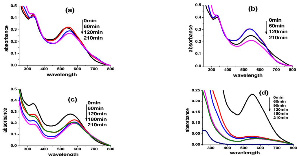
Fig.5. U.V-visible spectra of (a) EBT aqueous solution, (b) EBT+H<sub>2</sub>O<sub>2</sub>, (c) EBT+BiVO<sub>4</sub> and (d) EBT+H<sub>2</sub>O<sub>2</sub>+BiVO<sub>4</sub> as a function of irradiation time (EBT-20ppm, BiVO<sub>4</sub>-100mg, H<sub>2</sub>O<sub>2</sub>-10μm)
