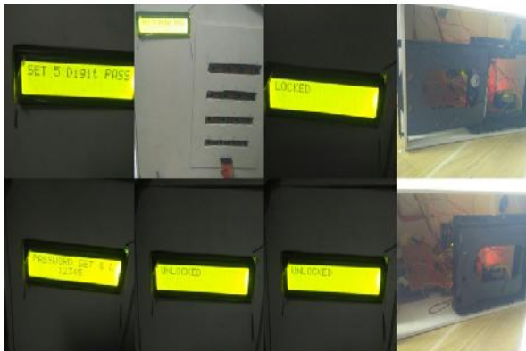
Fig 6. Digital locking system with keypad matrix and real time operation of digital locking system
