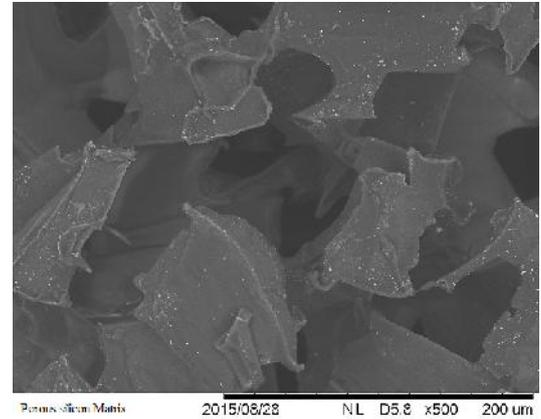
**Figure 9** Scanning electron microscope image from porous silicon matrix, cross-section the shows pore connections and density.
