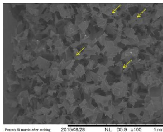
**Figure 4** Porous silicone matrix after etching process.
