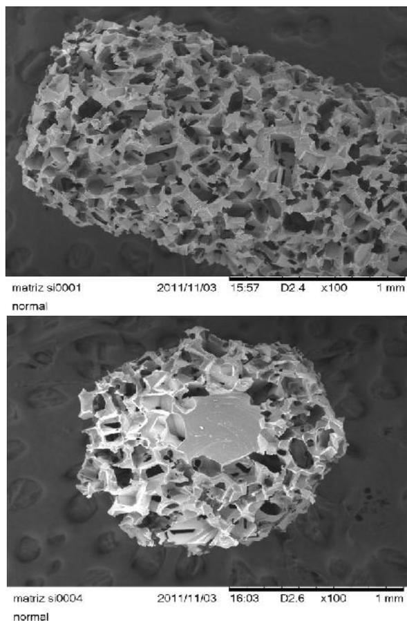
**Figure 1** Porous silicon matrix made with the use of pore forming agent, SEM imaging 100X.
