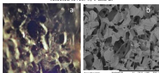
**Figure 7** Uncoated porosity silicone matrix obtained using the technique of leaching, a: 125X magnification, SmartScope Flash 200, optic machine, b: SEM 180X.
