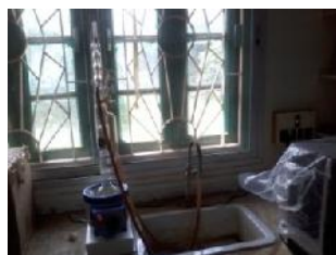
Fig. 1. Preparation of plant extract by using Soxhlet apparatus
