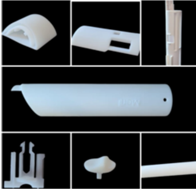
Figure 2 3D printed parts of the biopsy gun prototype before assembly and testing.
