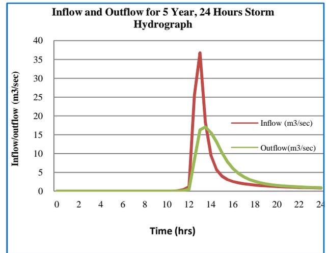
Figure 7 Inflows and Outflow for 5 Year, 24 Hours Storm Hydrograph at Detention Basin.
