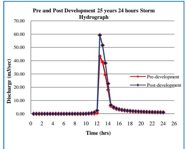
**Figure 2** Pre and Post Development 25 Years, 24 Hour Design Hydrograph
