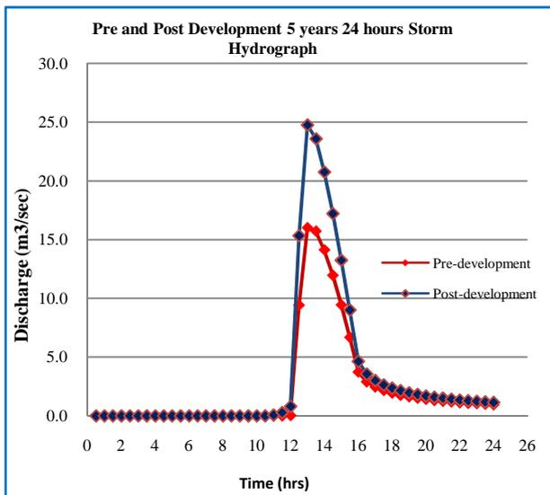
**Figure 1** Pre and Post Development 5 Years, 24 Hour Design Hydrograph.
