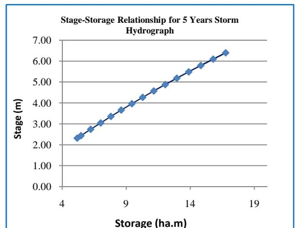
**Figure 4** Stage-Storage Relationship to Handle 5 Year, 24 Hour Runoff
