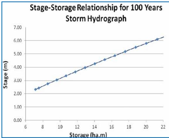
Figure 6 Stage-Storage Relationship to Handle 100 Year, 24 Hour Runoff
