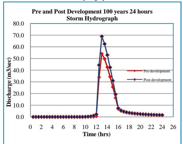
**Figure 3** Pre and Post Development 100Years, 24 Hour Design Hydrograph.
