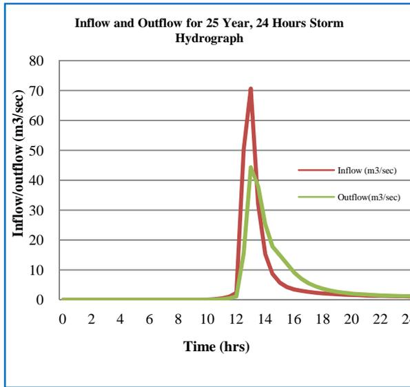
Figure 8 Inflow and Outflow for 25 Year, 24 Hours Storm Hydrograph at Detention Basin.
