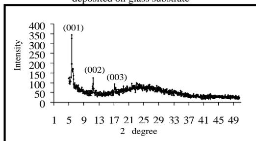
Figure 5 XRD pattern of the pentacene thin film (annealed in vacuum at 100°C) deposited on glass substrate
