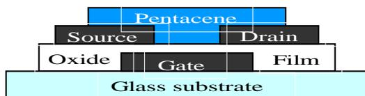
Figure 2 Structure of the OTFT
