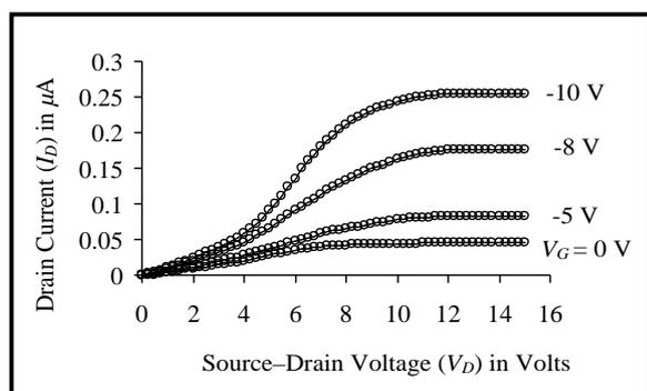
Figure 6 Plots of drain current  $I_D$  vs. source-drain voltage  $V_D$  at various gate voltages  $V_G$
