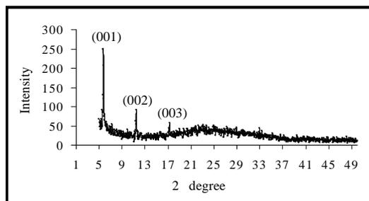
Figure 4 XRD pattern of the pentacene thin film (not annealed) deposited on glass substrate
