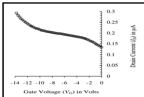
Figure 7 Plots of drain current  $I_D$  vs. gate voltage  $V_G$  at constant source-drain voltage  $V_D = 4$  volts
