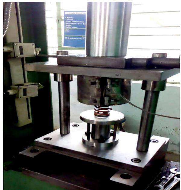
**Fig 3** Die with heater setup
