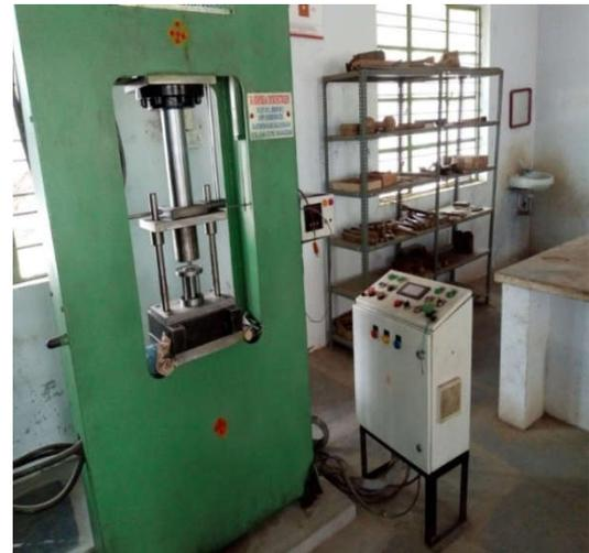
**Fig 2** Hydraulic deep drawing machine
