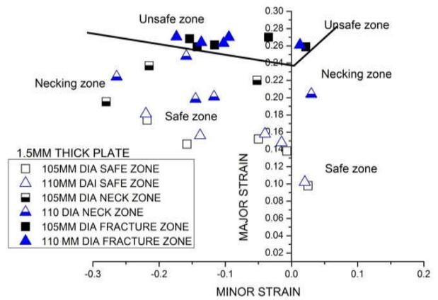
Graph 9 FLD for 1.5mm thick sheet
