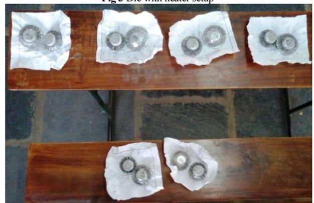
Fig 4 Drawn cups with different thickness
