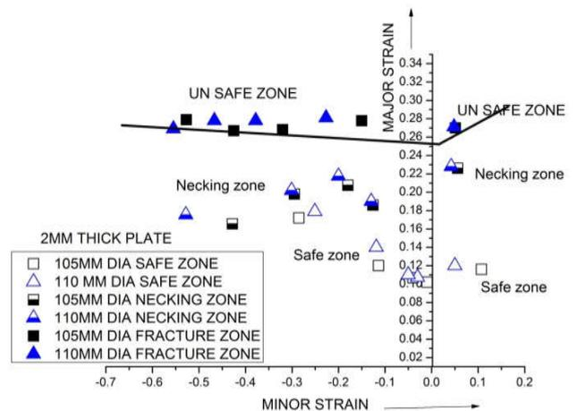
Graph 10 FLD for 2mm Thick sheet
