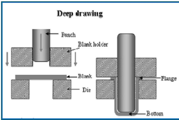
**Fig 1** Deep drawing of cylindrical cup formation
