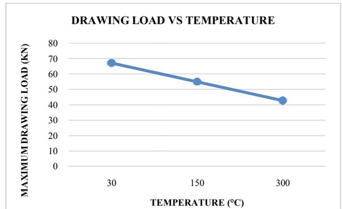
Graph 1 Maximum draw load at various processing temperatures
