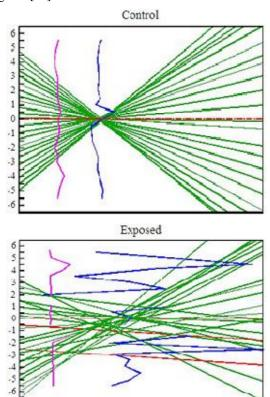
Fig. 2 - Left - Good quality lens - all rays passing through the lens have similar focal length. Right - Exposed lens, showing considerable variability in the focal length of the beams passing through the lens.
