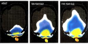
Fig. 1 - Absorption of electromagnetic radiation from a cell phone based on age (Frequency GSM 900 MHz)
