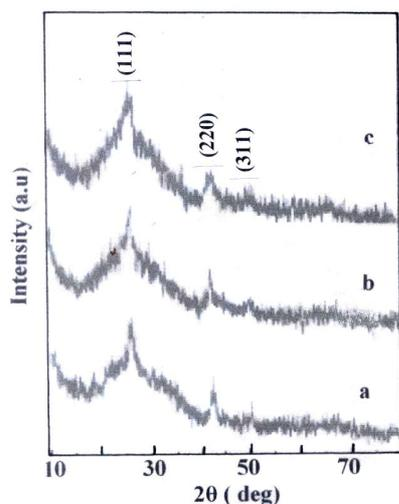
Fig.1 X-ray diffraction pattern of CdSe films deposited at different duty cycles (a) 50 % (b) 33 % (c) 15 %
