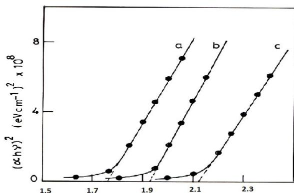
Fig.3 Variation of band gap with wavelength for CdSe films deposited at different duty cycles (a) 50 % (b) 15 % (c) 6 %
