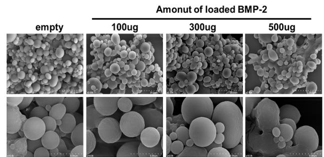
Fig 1 SEM micrographs of chitosan microspheres loaded with BMP-2 with different protein contents.
