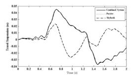
Figure 22 Suspension deflection for second road input
