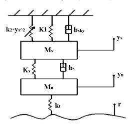
Figure 2 Suspension System Combined with Nonlinear Energy Sink and Skyhook
