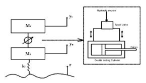
Figure3 Quarter Car Model with Hydraulic System
