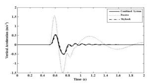
Figure19 Vertical acceleration for first road input
