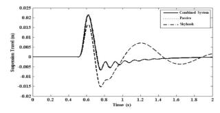
Figure21 Suspension deflection for first road input
