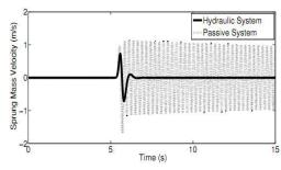
Figure7 Car Body Velocity
