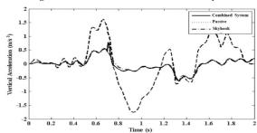
Figure 20 Vertical acceleration for second road input
