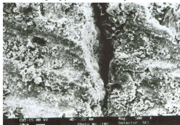
Fig 2 SEM microphotograph showing silver amalgam restoration-tooth interface with marginal gap formation at 500X magnification
