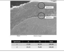
Figure 8 EDS-EDX analysis of the magnetite patina
