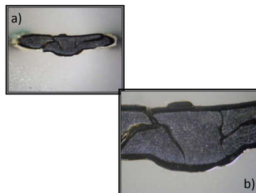
Figure 6 a) Segment of the rivet cut by a longitudinal plane, protected by the patina of magnetite. b) Detail of figure.6a
