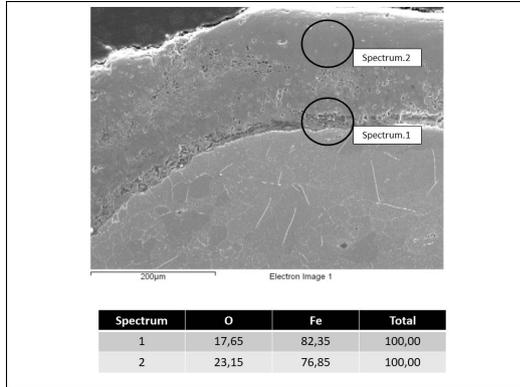
Figure 8 EDS-EDX analysis of the magnetite patina
