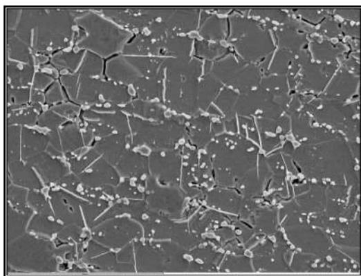
**Figure 11** SEM image of the steel microstructure of the ring. Globulized iron carbides and Widmanstätten acicular cementite are observed in a ferrite matrix.
