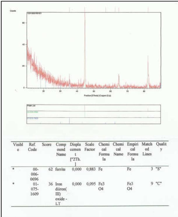
Figure 7 Diffractogram of the magnetite patina
