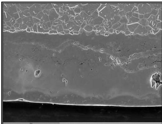
Figure 9 SEM image showing the fairly compact and homogeneous and continuous thickness of magnetite patina
