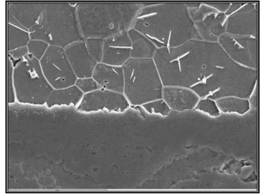
Figure 10 SEM image showing the good adhesion of the magnetite patina with the steel substrate
