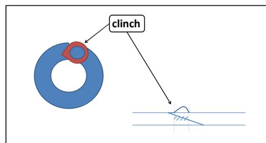
Figure 3 Schematic drawing of one of the rings of the mesh fragment with the crushing of the ends and the rivet
