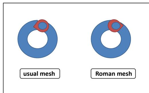
Figure 4 Schematic drawing of chain mail rings according to the Roman model and the usual one. In our fragment of mesh dimension the model presented is the usual one.
