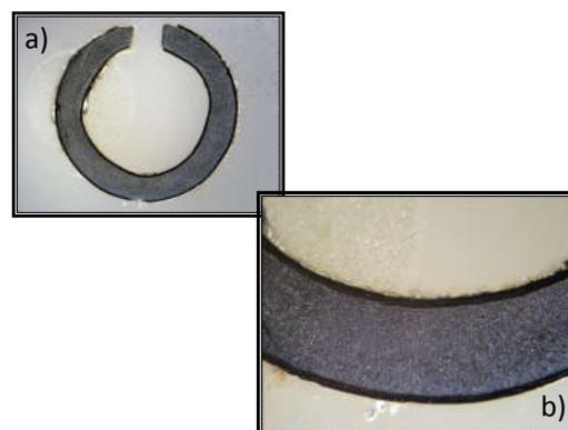
Figure 5 a) Ring belonging to the fragment of mesh with the segment of the rivet cut, protected by the patina of magnetite. b) Detail of figure 5a.
