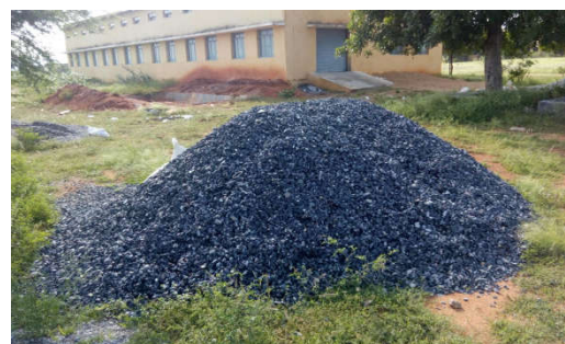
Marble stone waste aggregate
