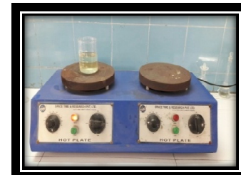
Carbopol is added and heated for 20 mts
