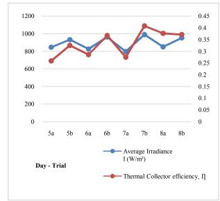
Fig 7 Variation of average irradiance and thermal collector efficiency for four days (with partition setup)
