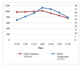
Fig 5 Variation of solar irradiance and outlet temperature with time for day 5 trial 2
