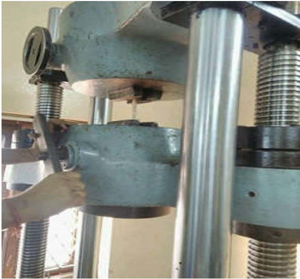
Fig 4 UTM machine Sample loaded condition for tensile testing.
