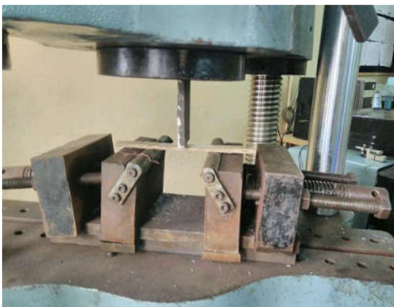
Fig 5 UTM machine Sample unloaded condition for Flexural testing.
