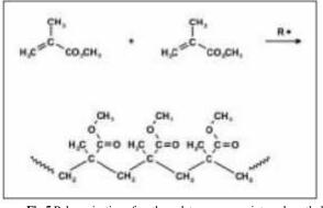
Fig 5 Polymerization of methacrylate monomers into polymethyl methacrylate
