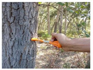
Figure 1 Operation of measurement of the thickness of the cork.
