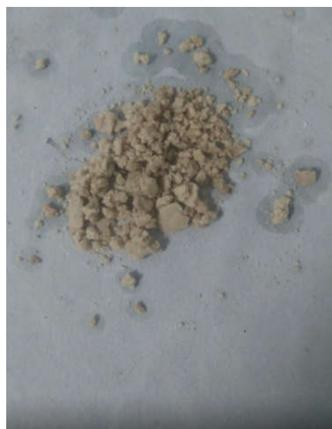
c) Crystallized and colour changed zeolite
