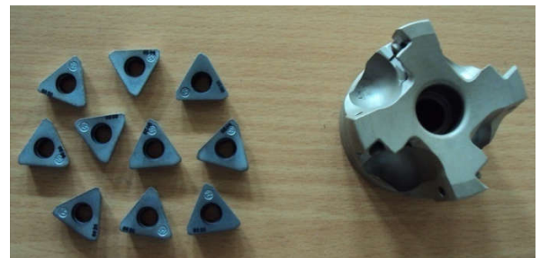
Figure 2 Cutting inserts and the milling cutter
