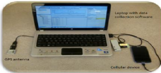
Figure 4 QoS test equipment setup
