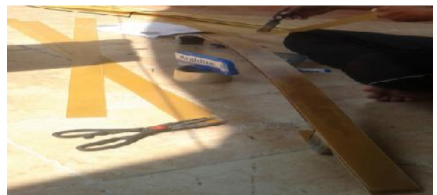
Fig. 3 Fabrication of composite leaf spring
