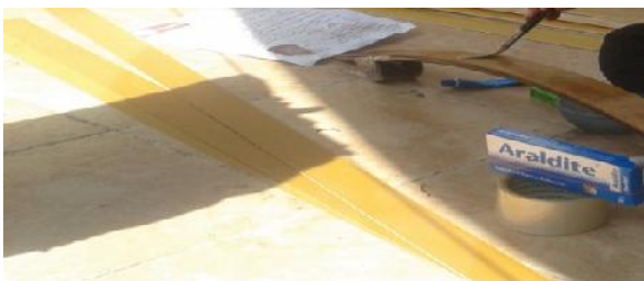
Fig.1 E glass / Epoxy Sheet of 0.5 mm thickness
