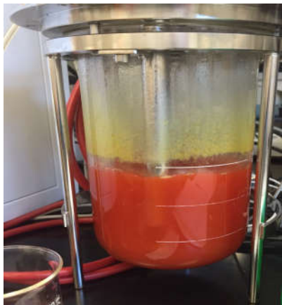
Figure 2 1.5 L bioreactor containing phase- I Photorhabdus luminescens
