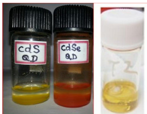
Figure 4 The as prepared QDs and CH 3 NH 3 SnCl 3 perovskite
