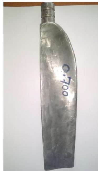
Fig.2 Blade made of pure aluminum
