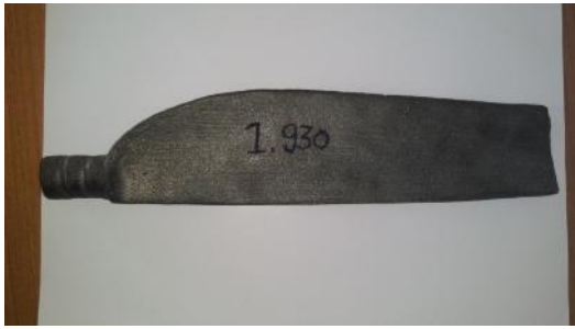
Fig.3 Blade made of Grey cast iron
