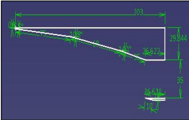
Figure 7 Rounded leading edge with three ramps and without deflection
