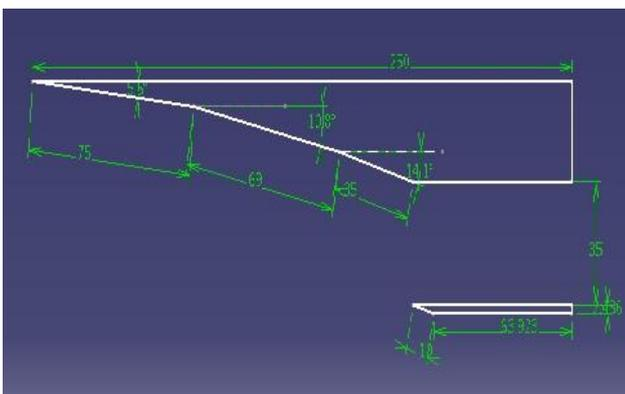
Figure 8 Four Ramped Inlet model with deflection
