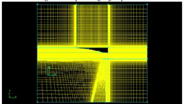
**Figure 17** Two Ramped Inlet model without deflection
