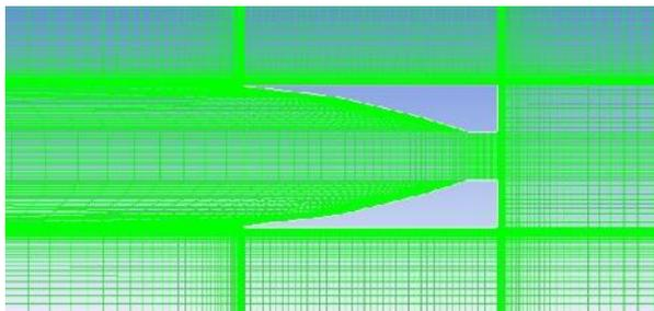
Figure 20 Mesh of axisymmetric scramjet inlet
