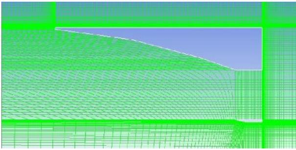
Figure 18 Mesh of scramjet inlet
