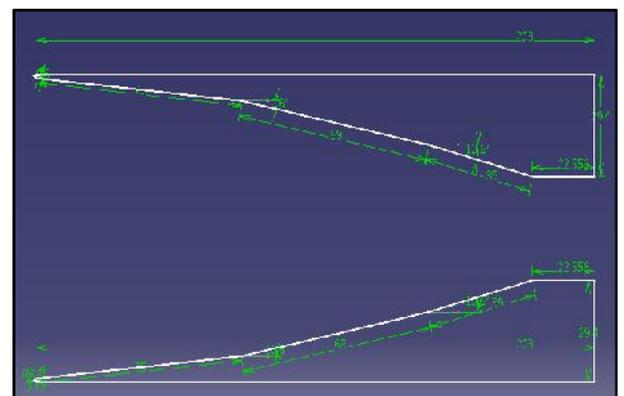
Figure 11 Axisymmetric Inlet model with rounded leading edge
