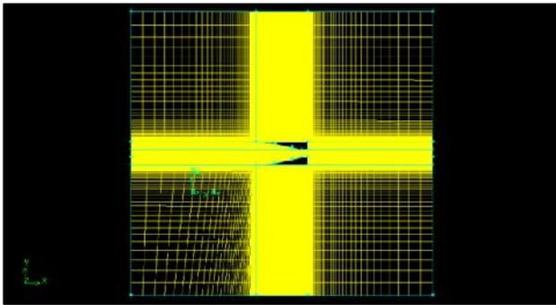
Figure 19 Axisymmetric Inlet model with rounded leading edge
