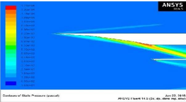
Figure 42 Pressure Contour
