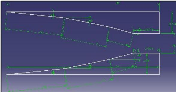
**Figure 12** Axisymmetric Inlet model with sharp leading edge
