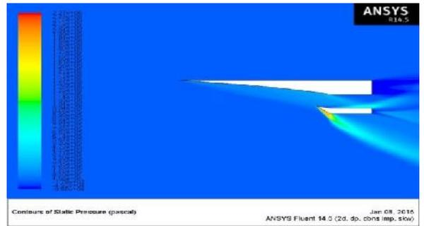
Figure 27 Pressure Contour
