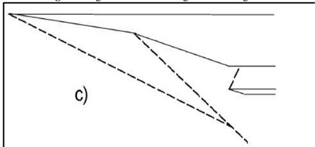
Figure 6 Flight Mach number lower than design one
