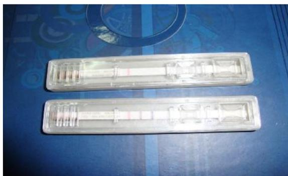
A positive reaction was identified by the presence of two rose-pink colour bands at the control (C) and test (T) labels. A visible rose-pink label at the control (C) label only was indicative of a negative reaction.
