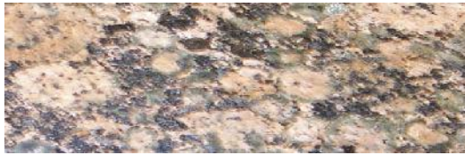
Figure 6 Size between 5 to 10 mm Tropic Brown rain-igneous rock with similar tissue containing a variety of crystal
