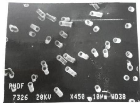
Figure 16 Plastic replication of microtubules scanned under SEM of PVDF
