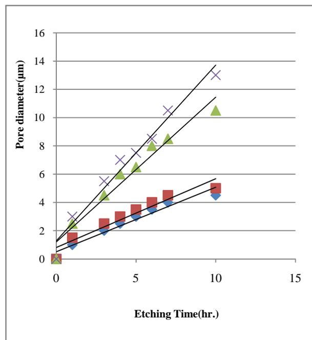
Figure 1 Variation of pore diameter with etching time for  $^{132}\text{Xe}$  (14.5 MeV/u) at various temperatures of the etching solution in Makrofol-KG
