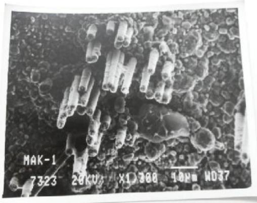
Figure 11 Microstructure (scanned by SEM) ensembles of Cu grown electrochemically through single-pore and multipore filters of Makrofol-KG
