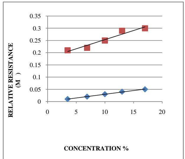
**Figure 8** Variation of change in resistance with concentration using single pore filter for *E. coli* and *C. bacillus* in water
