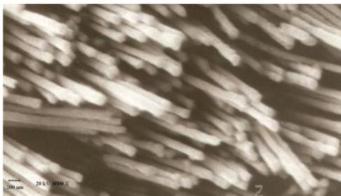
Figure 13 SEM Photograph of copper nanowires of 200nm diameter grown by electrodeposition in AAM<sup>25</sup>.
