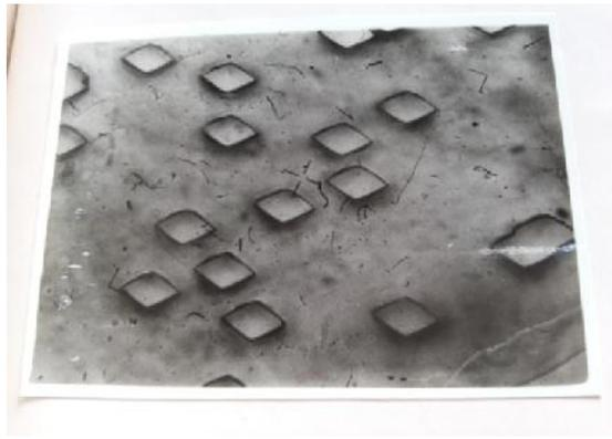
**Figure 4** Photomicrograph of  $^{132}\text{Xe}$  (5.9 MeV/u) ion track pores (major axis  $\sim 26.9 \mu\text{m}$  and minor axis  $\sim 17.71 \mu\text{m}$ ) in muscovite mica
