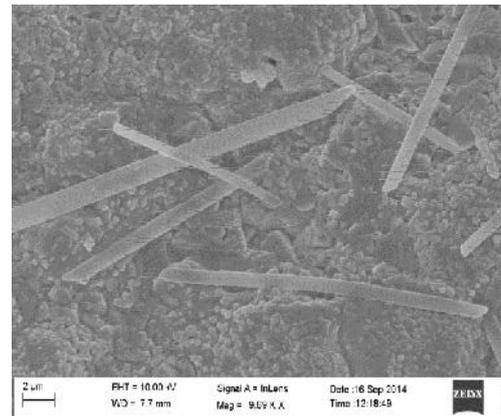
Figure14 SEM Photograph of copper nanowires of 250nm diameter grown by electrodeposition in makrofol- KG.
