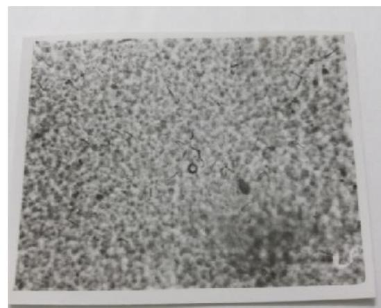
Figure 3 Photomicrograph of  $^{132}\text{Xe}$  (14.5 MeV/u) ion track singlepore (2µm) in Makrofol-KG
