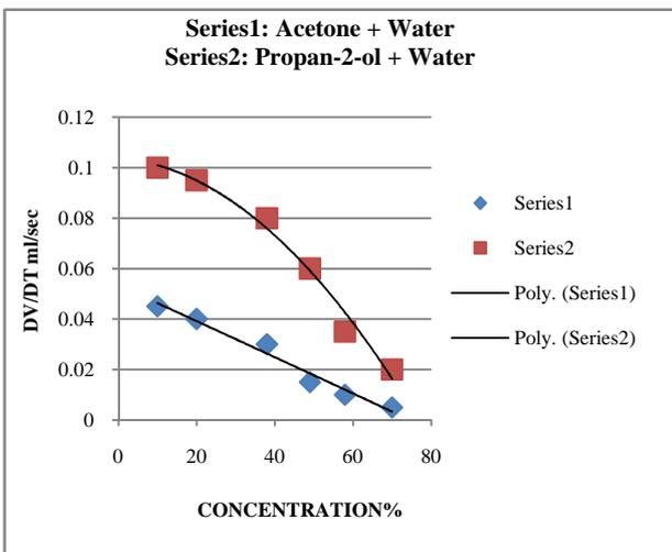
**Figure 7** Variation of flow rate,  $dV/dt$  with concentration of solutes in water at a constant pressure difference
