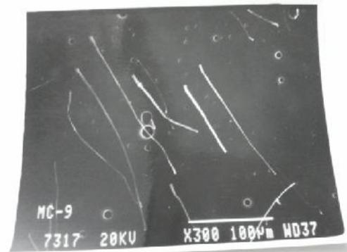
Figure15 Plastic replication of microtubules scanned under SEM of Kapton
