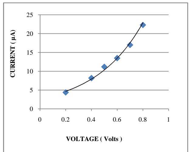
**Figure 10** V-I variation observed in nanopores using polluted water
