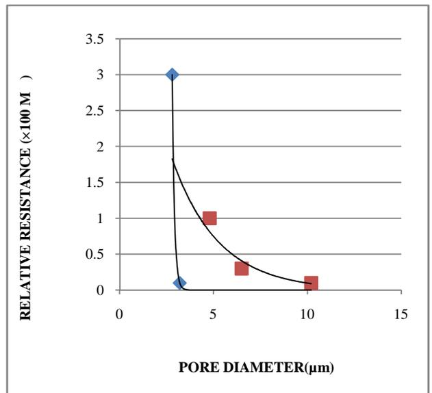
**Figure 9** Variation of change in resistance with pore diameter for *E. coli* and *C. bacillus* in water
