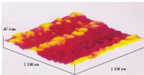
Figure 12 AFM image of 3-dimensional ensemble of Cu-Se grown electrochemically using ITFs of Makrofol-KG
