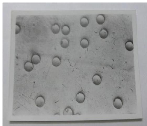
Figure 2 Photomicrograph of  $^{132}\text{Xe}$  (14.5 MeV/u) ion track multipores (~21.68 µm)
