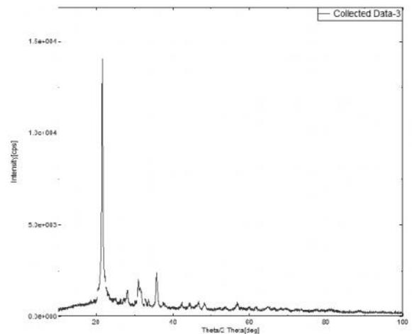
Graph 2 X-ray diffraction pattern of synthesized SiC nano-powders after heat treatment at 850°C.
