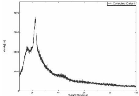
Graph 1 X-ray diffraction pattern of synthesized SiC nano-powders, dried at 180°C for 1 hours.
