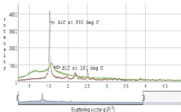
Graph 3 Comparison spectra of SiC at 180°C and at 850°C. From the above comparison spectra we concluded that synthesized SiC nano powder was amorphous in nature initially at 180°C. After the heat treatment of synthesized SiC nano powder at 850°C clearly shows the crystalline nature.
