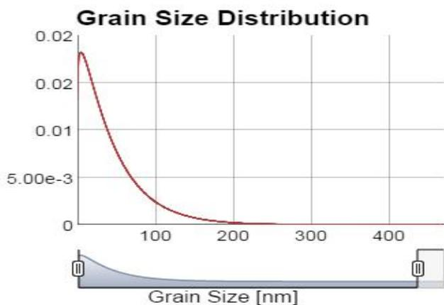
Graph 4 Grain size distribution curve. Average size distribution of synthesized SiC nano powder found to be 35-40nm.
