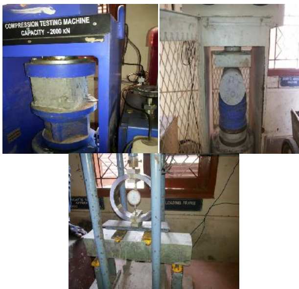
Fig. 1 Compression, Split Tensile and Flexural Strength Testing Set ups
