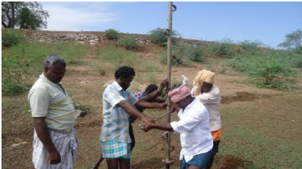
Figure.1 Sampling in Lake by Rotatory Drill.
