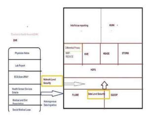
The Secured Big Data architecture of healthcare is shown in figure 1. Electronic health record is a heterogeneous data set which is given as input to HDFS through flume and sqoop. Analysis on the data is performed using Map-Reduce and HIVE by implementing machine-learning algorithms which
