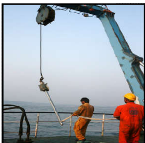
Figure 1 Process of sediment core retrieval by the gravity corer onboard Sagar Manjusha cruise
